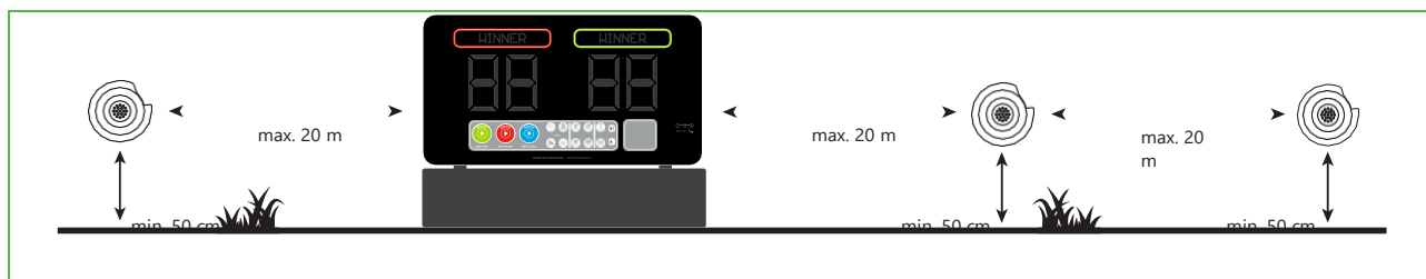
Figuur 6 The maximum distance between parts
